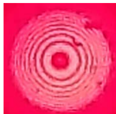
Fig. 2. Interference fringe captured from smartphone reader. Used to calculate IOP.
